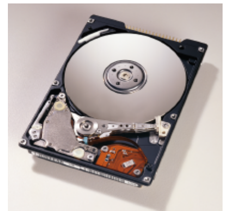
Hitachi Travelstar 40GN: 9.5mm, 4,200rpm, 40GB ATA-5 hard disk drive 1
