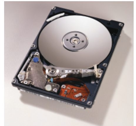
Hitachi Travelstar 60GH: 12.5mm, 5,400rpm, 60GB ATA-5 hard disk drive 1
