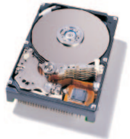
Travelstar 8GS 2.5-inch 8.1 GB, 17 mm hard disk drive
