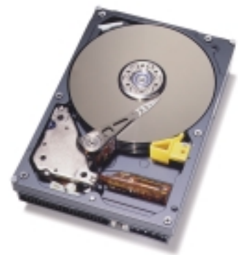
IBM Deskstar 34GXP 3.5-inch 7200 RPM 34.2, 27.3, 20.5, and 13.6 GB low-profile ATA disk drive
